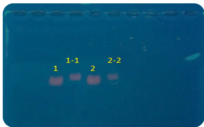
Fig. 3. Gel electrophoresis of dsDNA-AgNCs formed by incubating DNA-AgNCs with (1) mutant type and (2) wild type target, and QDs@dsDNA-AgNCs formed after mixing QDs solution with (1-1) mutant type and (2-2) wild type dsDNA-AgNCs.
