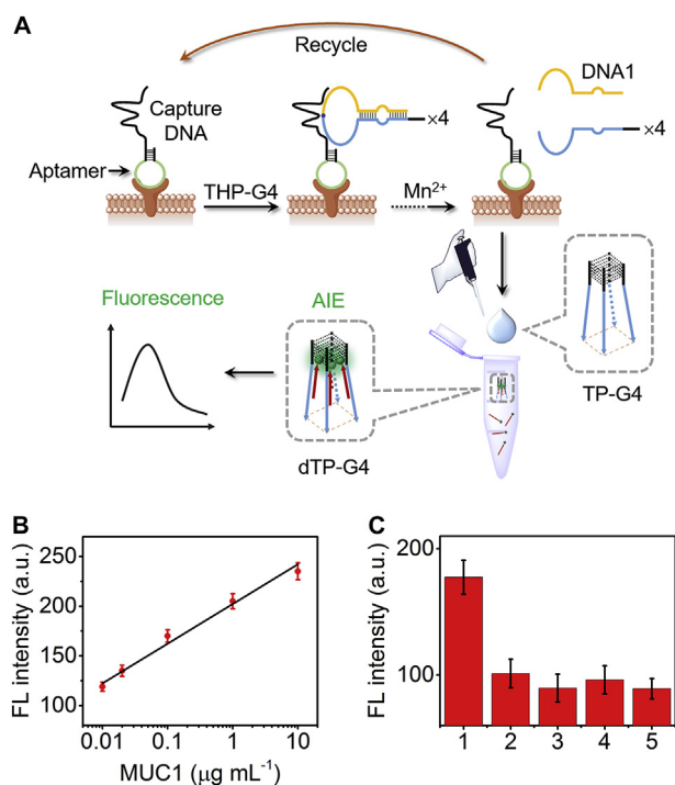
Fig. 4. (A) Schematic illustration of controlled assembly of AIEgens triggered by DNAzyme for detection of plasma membrane proteins. (B) Fluorescence calibration curve for detection of MUC1 protein. (C) Fluorescence results of the proposed strategy for detection of MUC1 on MCF-7 (1) and MDA-MB-453 (2) cells, and control experiments on MCF-7 cell labelling with aptamer (3), DNAzyme (4), aptamer-T37 (5).
